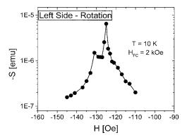
FIG. 4. Applied field dependence of the magnetic viscosity on the left side of the hysteresis loop at  $T=10\,\mathrm{K}$  and  $H_{\mathrm{FC}}=2\,\mathrm{kOe}$ . The solid line is a guide to the eye. Note that this figure and Fig. 3 are plotted over the same range in S and over the same field range of 70 Oe allowing easy comparison.
