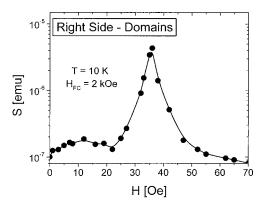
FIG. 3. Applied field dependence of the magnetic viscosity on the right side of the hysteresis loop at T = 10 K and  $H_{FC} = 2 \text{ kOe}$ . The solid line is a guide to the eye. Note that this figure and Fig. 4 are plotted over the same range in S and over the same field range of 70 Oe allowing easy comparison.
