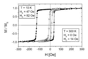
FIG. 1. Magnetization hysteresis loops taken at 300 K (open circles) and after cooling in a field  $H_{\rm FC}$ =2 kOe to 10 K (solid circles). The data are normalized to the saturation magnetization  $M_S$ . The values of  $H_E$  and  $H_C$  are displayed for the two curves.
