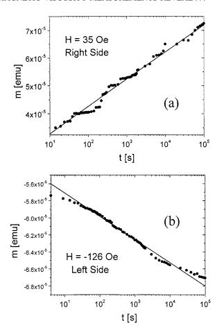
FIG. 2. Time dependence of the magnetic moment m at  $T=10 \, \mathrm{K}$  for the right and left side of the hysteresis loops after cooling in a field  $H_{\mathrm{FC}}=+2 \, \mathrm{kOe}$ .  $H=+35 \, \mathrm{Oe}$  in (a) and  $-126 \, \mathrm{Oe}$  in (b). The solid lines are fits to Eq. (3) to obtain the viscosity S. A field of magnitude 500 Oe was used to saturate the films before measurement of the time dependence.
